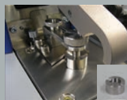
Adapter for wires with a diameter of 1-3 mm
